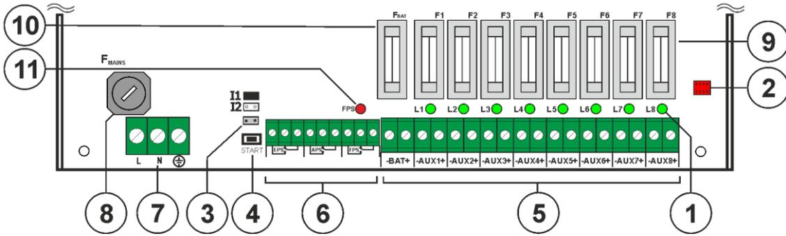
Fig. 2b. View of power supply module HPSCDG2-12V8x1A
